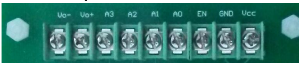
Fig2 terminals of watermeter DEMO
